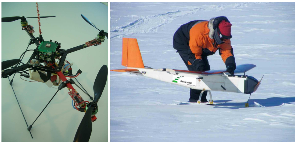
Figure 2.1: UAVs under development at the Geospatial Research Centre, University of Canterbury, for which positioning is useful include this quadrotor (photo by John Stowers), and this remote-controlled fixed-wing UAV designed for the Antarctic, images from which are used in Chapter 10.1 (from Barnsdale, 2010).
