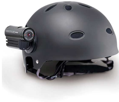
Figure 2.5: Contour HD wearable camera. This rugged helmet-mounted camera with a 135 degree FOV weighs 116g, currently costs around US$250, and has a battery/recording life of about 2 hours. Images from this camera are used to test BoWSLAM, as described in Chapter 8.
