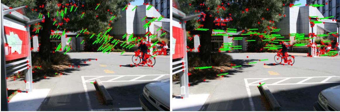
Figure 7.4: BaySAC successfully avoids outlier correspondences from moving objects. The red dots indicate detected features, and the green lines indicate the locations in the previous frame which features are matched to. Despite the high density of features on the cyclist, following BaySAC no matches are found here.
