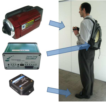
Figure 2.4: One potential use for SLAM is as a pedestrian navigation aid. This vision-aided pedestrian navigation system combines computer vision with measurements from a IMU, and from GPS when available. A Sony Handycam DCR-SR47 is used to collect images, and a low-cost Microstrain 3DM-GX1 IMU is mounted to the pedestrian’s foot (from Hide et al., 2009).
