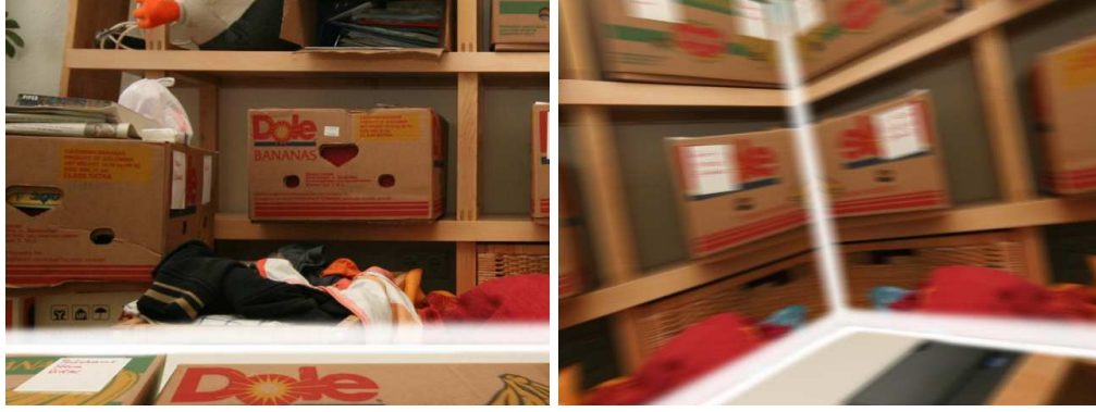
Figure 8.14: Simulated frames from the SLAMDUNK dataset with added motion blur, covering a small loop. The repeated image of banana boxes occasionally triggers false loop-closure.
