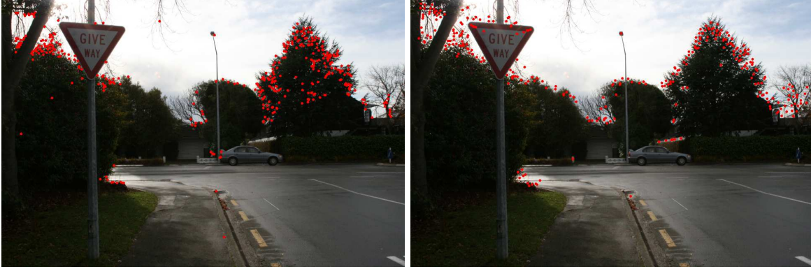
Figure 4.2: Top 380 interest points found by the FAST (left) and SURF’s DoH (right) feature detectors. Features are closely grouped around the most textured regions, potentially leading to poorly-conditioned geometry. Imposing a minimum separation constraint degrades repeatability (Section 4.4.1).
