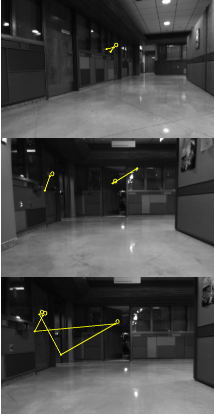
Fig. 3. Objects from the same class observed on several similar-looking doors, University of Alberta dataset. (Each object is measured in one place per pair of frames, however in BoWSLAM each frame is registered to many others, so the same type of object may be measured in several places in the same frame.)
