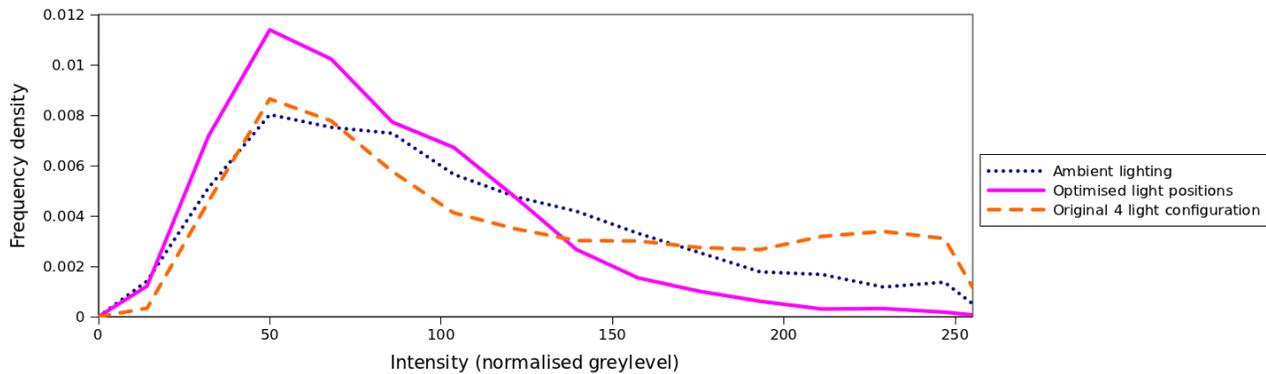
Figure 6. Variation in image intensity on vine pixels, with old and new lighting configurations, and under ambient light.
