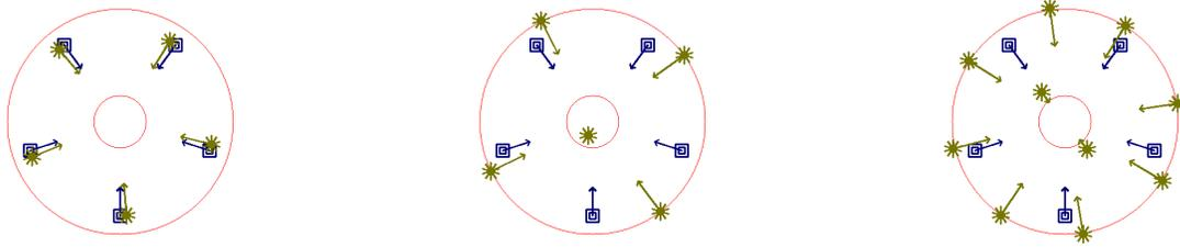
Figure 7. Lighting layouts for the DIET breast cancer screening system; orthographic view from above. The lights and cameras lie on a hemisphere, which is outlined with the large circle (30cm radius). The breast position is marked by the smaller circle. The original lighting configuration is shown on the left; the optimised configuration of five lights is shown in the middle, and an optimised configuration of 10 lights is shown on the right.
