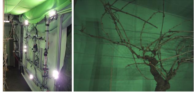
Figure 2. Lighting system deployed on a vine imaging robot, and a typical vine image.
