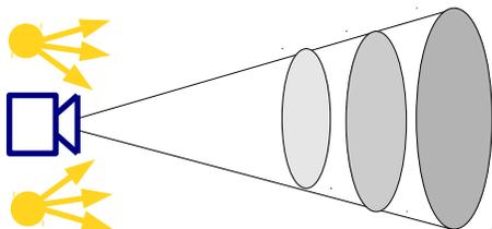
(c) When the DOF is large, light sources positioned near to the camera lead to large variation in light intensity at different depths.
