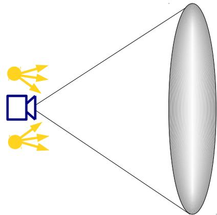
(b) When the FOV is large, typical light sources positioned near to the camera lead to an unevenly-illuminated scene, as points near the centre of the FOV are closer to the light, and are considerably brighter than points at the edge.
