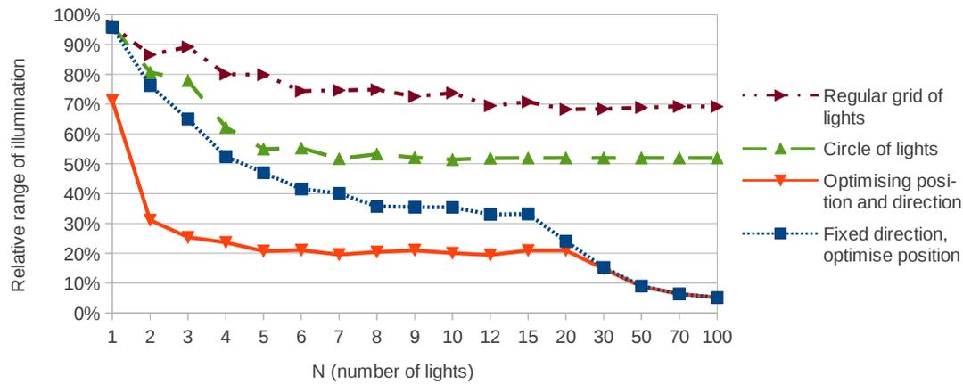
Figure 5. Relative range of illumination obtained for the vine imaging robot, with varying  $N$ . Lower values are best.
