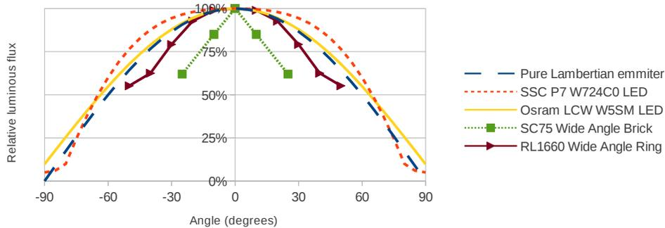
Figure 3. RCFs for some wide angle machine vision lights and LEDs.
