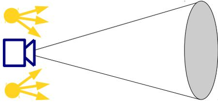
(a) When the FOV and DOF are small, an even lighting field can be obtained easily by positioning light sources close to the camera.
