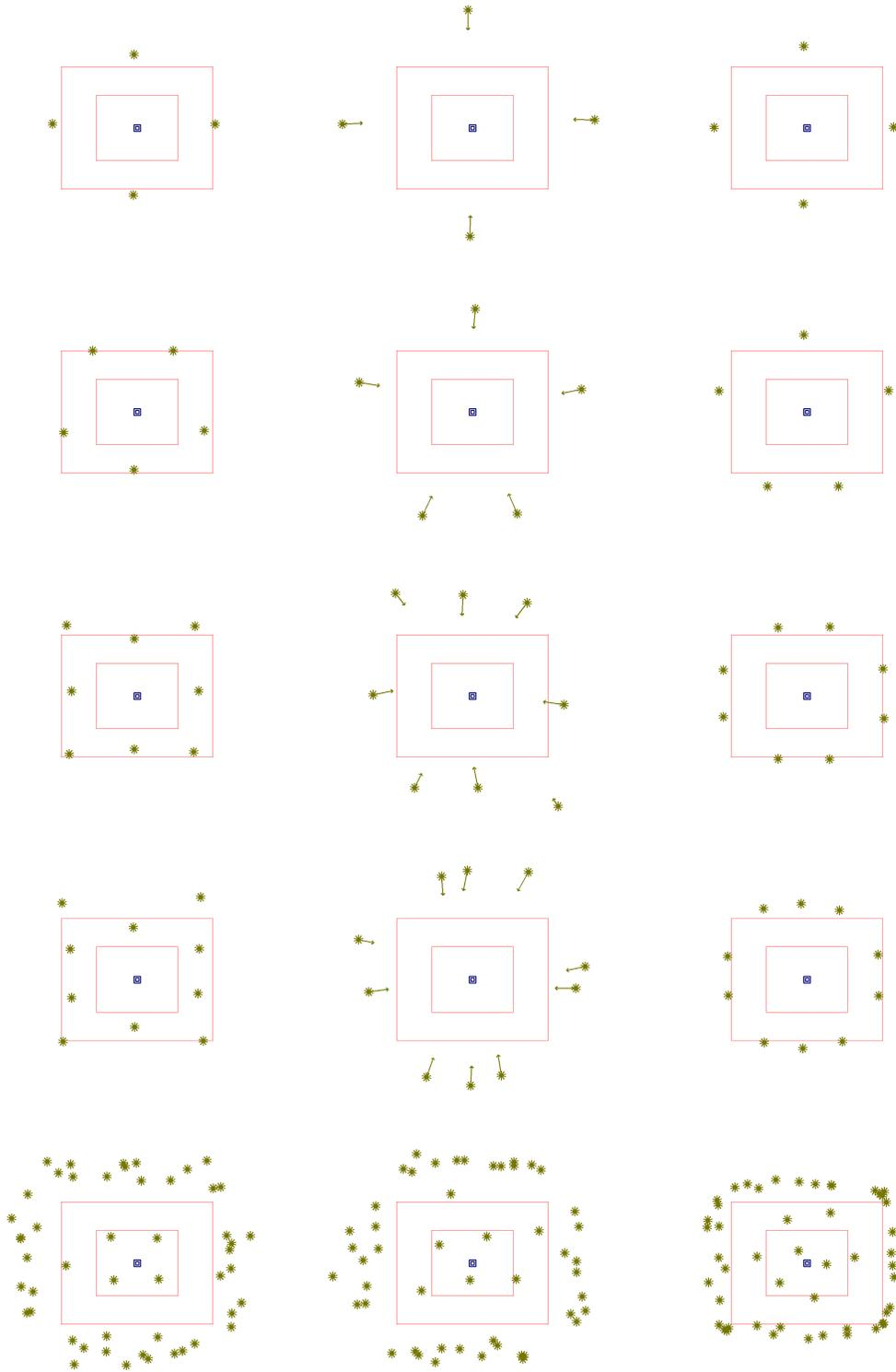
Figure 4. Lighting layouts for the vine imaging robot for  $N = 4, 5, 8, 10, 50$ . View from behind the front-pointing camera (small double-square), with the FOV at 35cm and 65cm marked with rectangles. Left: position front-pointing lights to minimise relative range; Middle: optimise positions and directions; Right: minimise range with occlusion.
