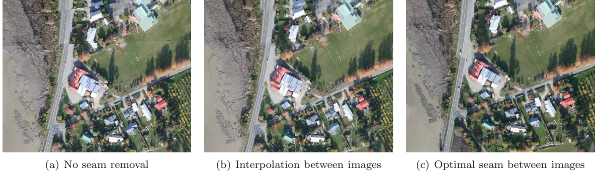
Figure 1: Simply warping images over each other leads to visible seams and broken edges when images do not quite align (a). The seams are successfully hidden by interpolating between frames, but artefacts around man-made straight edges still occur (b). An optimal seam between images usually removes both kinds of artefact (c).
