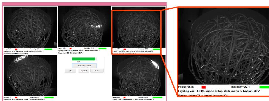
**Fig. 4.** The DIET machine’s GUI for setting camera focus. The wire ball has sharp edges at a range of depths. The focus and aperture are set to maximise the sum of squared differences between neighbouring pixels.
